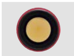
Standard lens showing browning after being subjected to gamma rays.
