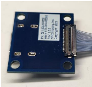
Figure 10. HDMI to KEL Adapter Back
