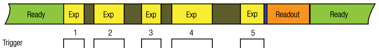
Figure 71: Multiple exposures - exposure time defined by trigger pulse length - number of exposures set to 5
