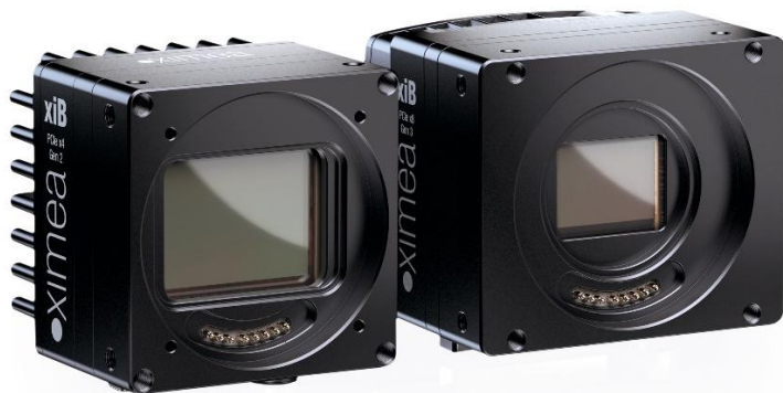
figure 2-1 xiB and xiB-64 camera with heat sinks.
