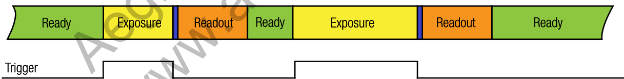
Figure 57: Exposure defined by trigger pulse length
