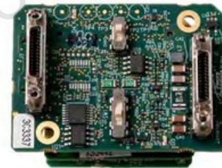
iPORT CL-U3-IND external Frame Grabber Oem Board Set (903-0020) for Camera Link Medium Mode
